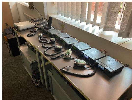
Figure 9: Radio base stations in the SOC connected to backup batteries stored in boxes
